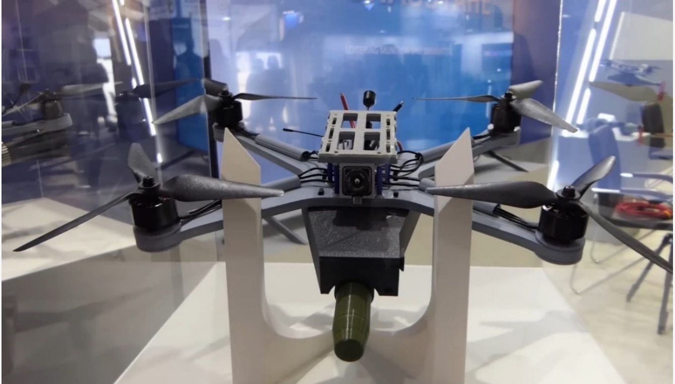
Fig 8: The Donaustahl MAUS FPV drone used for reconnaissance and strike missions
